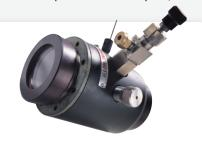
thermocouple port and vacuum valve. Windows are secured using threaded end caps and chemically resistant seals. The cells can be dismantled to allow easy cleaning and window replacement.
