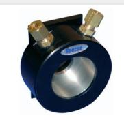
The Water Heating Jacket is similar to the Electrical Heating Jacket, but it uses circulating water to heat the sample cell. A jacket around the circular aperture is filled with a solution, for example water, heated by a thermocirculating system. Temperature control of the sample holder is reliant upon this thermocirculating system.
